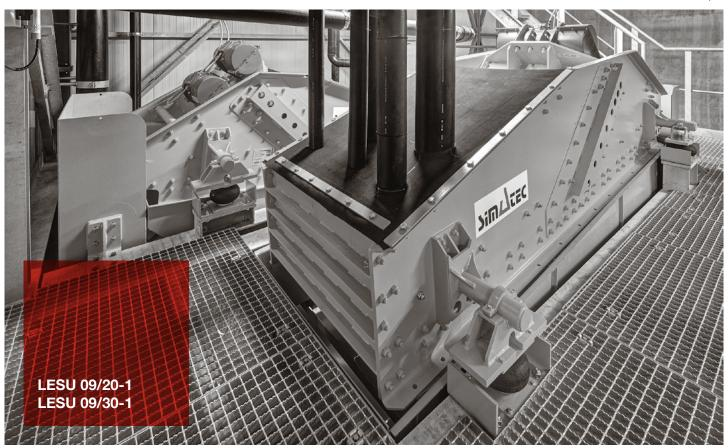
THE AIR SUSPENSION PROTECTS THE STEEL STRUCTURE, THE SCREENING MACHINE AND YOUR WALLET 400 MM PU IMPACT DECK FOR CAREFUL MATERIAL ADDITION AND DISTRIBUTION
